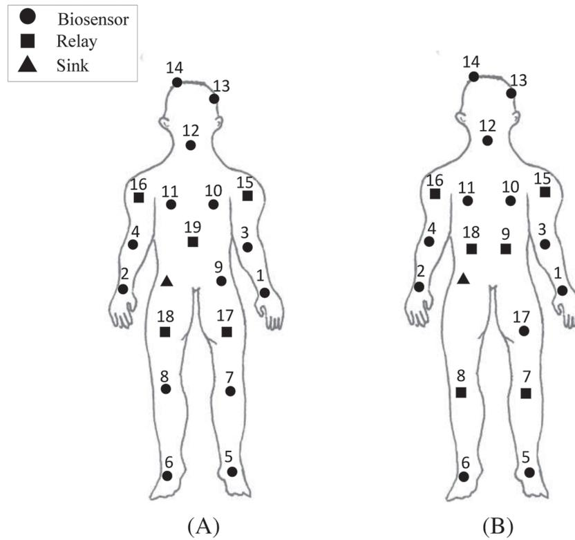
FIGURE 1 Applied layout for nodes in WBAN: (A) first layout and (B) second layout
