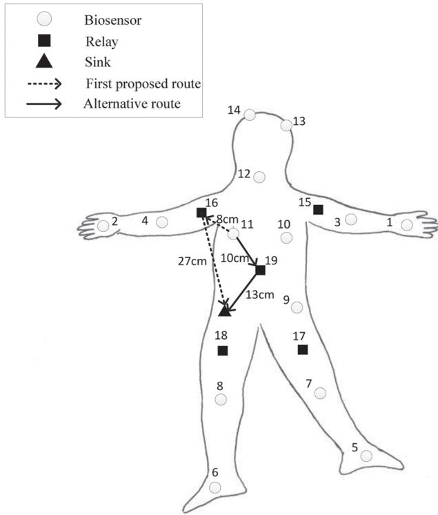
FIGURE 5 An example for relay selection in the first applied layout
