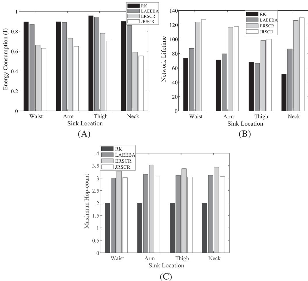
FIGURE 11 Network performance versus different sink locations: (A) energy consumption, (B) network lifetime, and (C) maximum hop count
