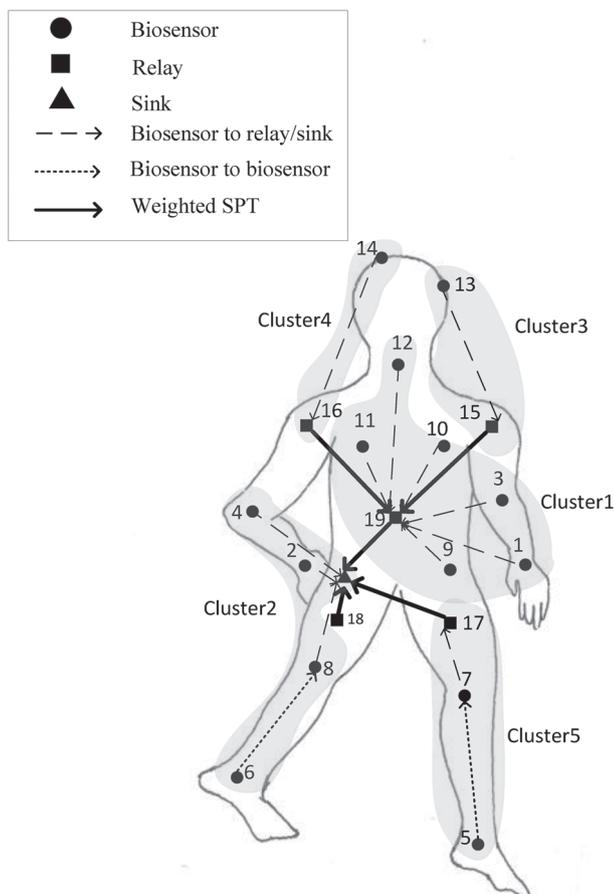
FIGURE 7 An example for clustering and routing in JRSCR
