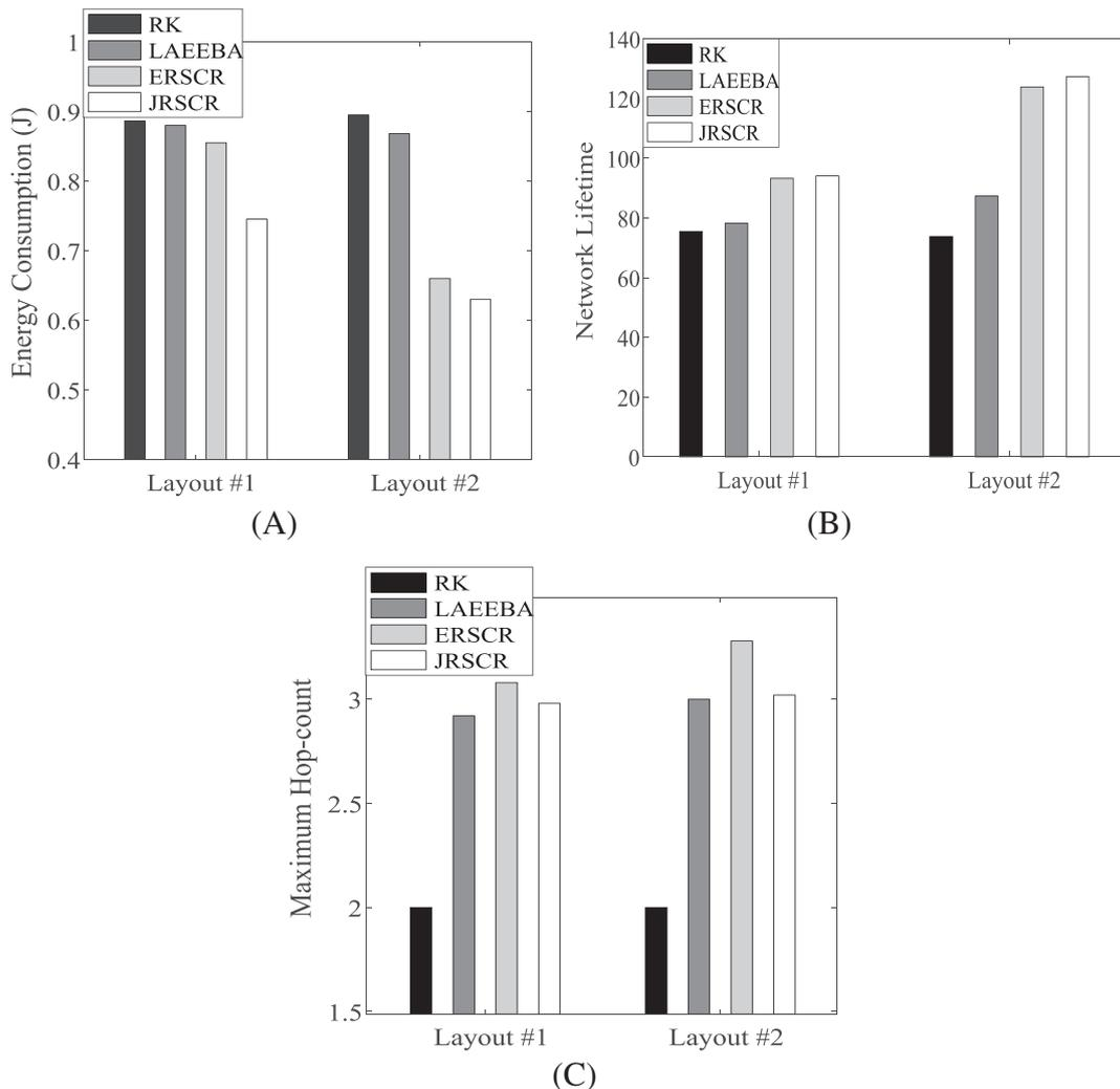
FIGURE 8 Network performance for two applied node layouts: (A) energy consumption, (B) network lifetime, and (C) maximum hop count
