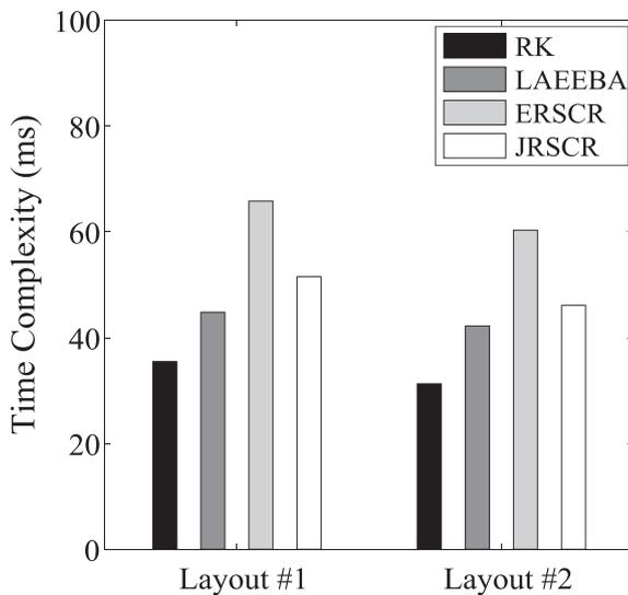
FIGURE 14 Time complexity for two applied node layouts
