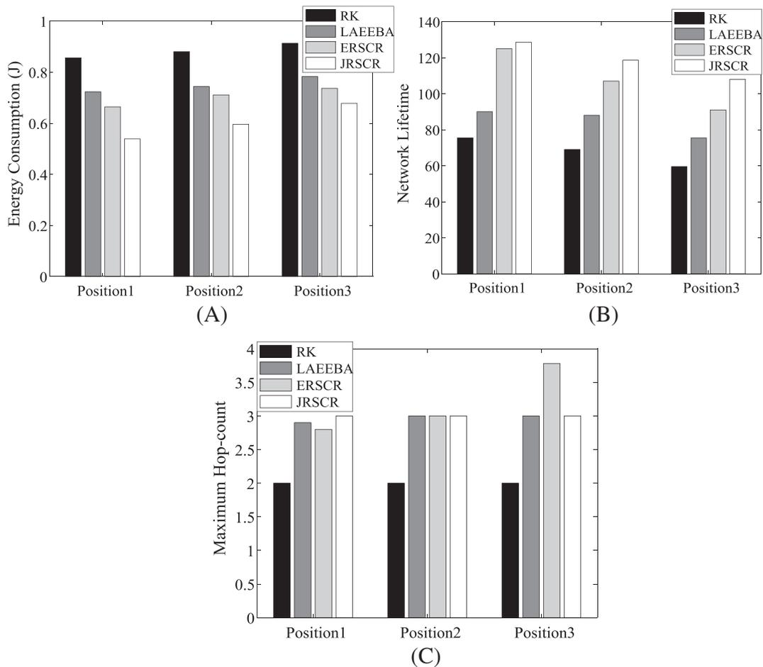
FIGURE 13 Network performance versus different body positions: (A) energy consumption, (B) network lifetime, and (C) maximum hop-count
