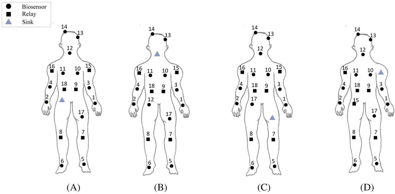
FIGURE 10 Different locations of sink in the second applied layout: (A) waist, (B) back of the neck, (C) left thigh, and (D) left arm
