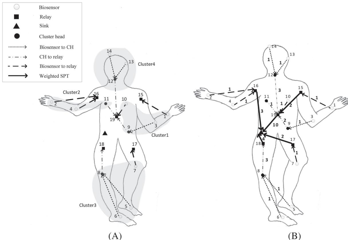
FIGURE 6 (A) An example for clustering and selecting the first forwarding node in ERSCR algorithm and (B) weighted SPT constructed between relays and sink node
