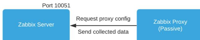
Figure 7.11 – Diagram showing passive proxy connection
